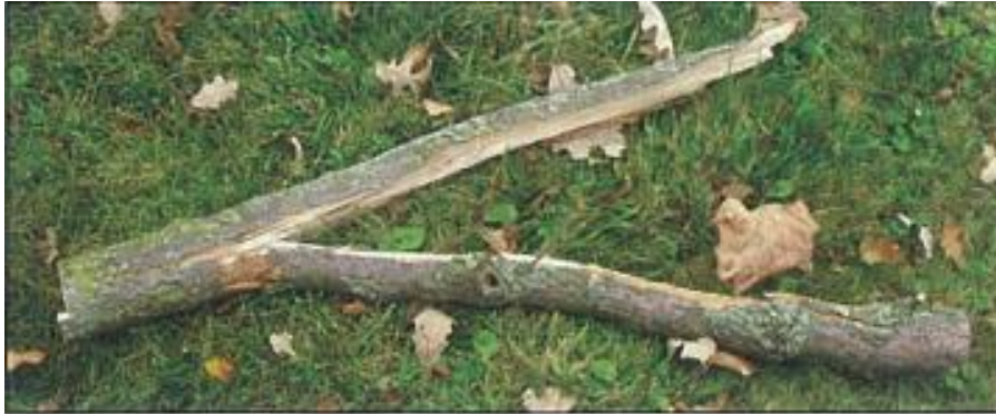
Moisture levels in EAB infested trees are lower and wood in those trees, upon breaking, has significantly more cracking.
