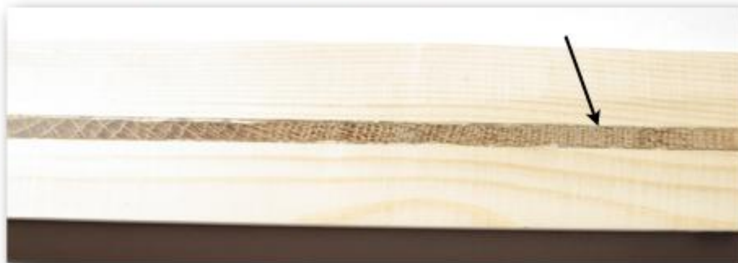
Above: Ash sample from a cut stump displaying very distinct annual rings. Below: Oak sample set into baton with tight rings (arrowed).
